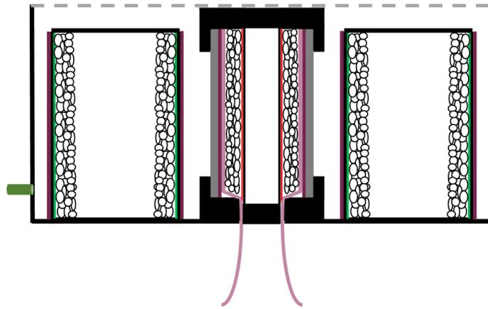
**Figure B-2:** Schematic of basic section of 122 L reactor (Anode-Cathode-Cathode-Anode)
