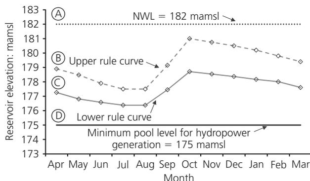
Figure 1. Pre-2002 rule curves for reservoir operation at Ubonratana reservoir (mamsl: metres above mean sea level; NWL: normal water level in reservoir)
