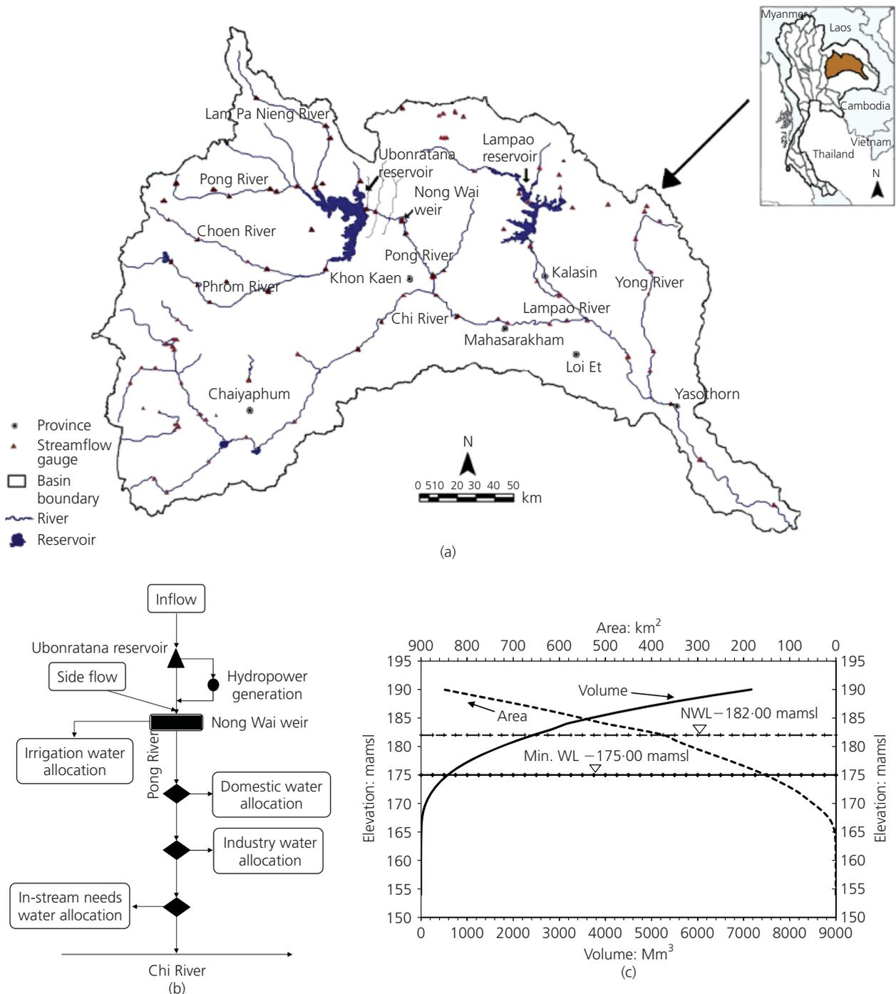
**Figure 2.** Study location showing: (a) map of Thailand, Chi River and the Mun River basins (Meethom, 2011); (b) schematic diagram of reservoir and the various diversions; (c) the reservoir elevation–area–storage relationship
