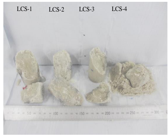
(b) failure surfaces of deformed samples
