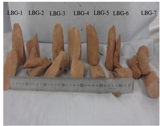
(b) failure surfaces of deformed samples
