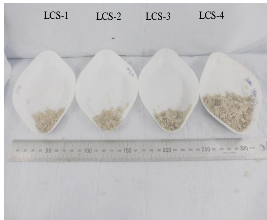
(c) debris recovered from failure surfaces of deformed samples
