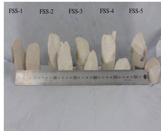
(b) failure surfaces of deformed samples
