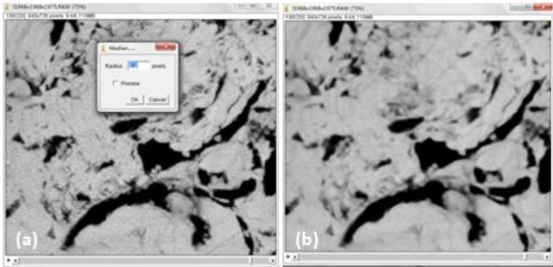
Figure B.5: The cropped images can be filtered by the median filter just set the radius of the filter. The effect of median filter can be shown in this figure. The noise which is the small points in (a) can be smoothed in (b).
